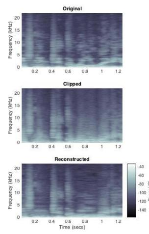
Figure 7: Clean, clipped, and reconstructed speech signal spectrograms.
