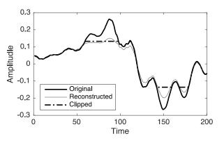
Figure 6: Clean, clipped, and reconstructed speech signal waveforms.
