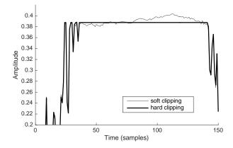
Figure 1: Soft clipping versus hard clipping.
