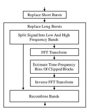
Figure 3: Block Diagram of sample replacement
