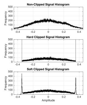
Figure 2: Histograms of clipped and non-clipped signals.
